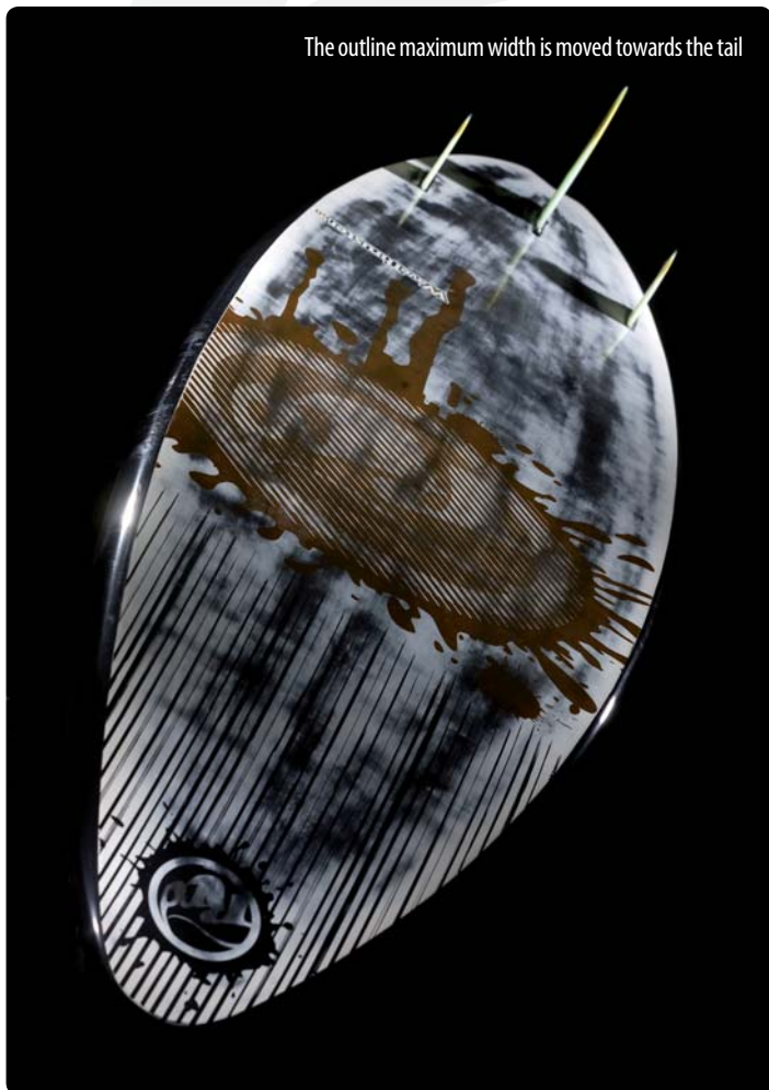
The curved outline tail design and the straight rocker with a simple V hull configuration
